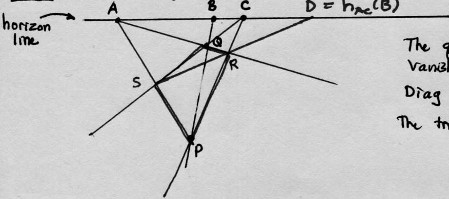
The quad PRQS has 2 sides going to vanishing pt A, and 2 to vanishing pt C
